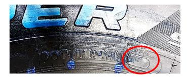
Only tires that exhibit the noncompliant (missing) date code on the white lettered side of the tire, are being recalled. Tires from the 5<sup>th</sup> week of 2025 (0525) that exhibit a compliant date code portion of the TIN are not subject tires and are not eligible for free replacement.
